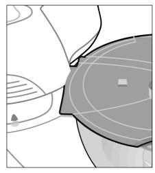
6 Turn the swivel head D clockwise and press to lock securely. Insert the glass bowl pusher N into the filler spout on the glass bowl lid G.
